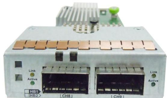
Figure 7 Rear view of Infortrend InfiniBand host board
